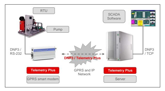
*Telemetry Plus* is a distributed software platform that provides reliable, efficient, and secure data transport between the field and the control room over the GPRS and IP networks.
